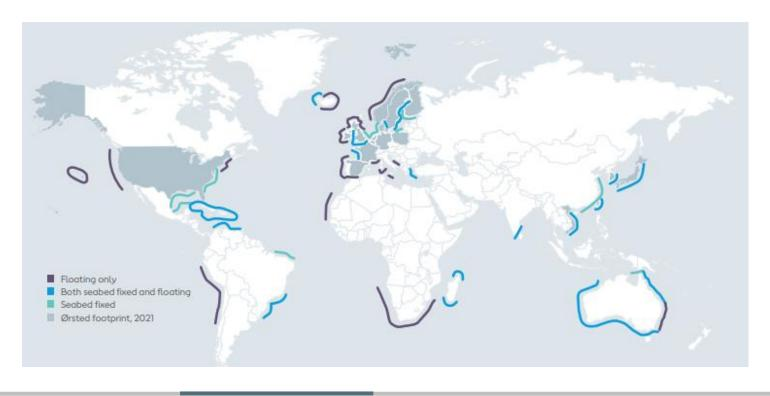
**80%** of total offshore generation potential is in waters deeper than 60 meters, which is beyond the feasible depth of most fixed turbines
