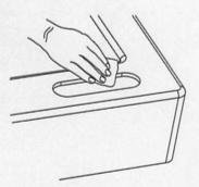
Do not touch the VHB tape after its protective sticker is torn off and avoid water or impurities stick to the tape. Please stick the panel to the tub firmly within 5 minutes after protective sticker of the tape is off.
