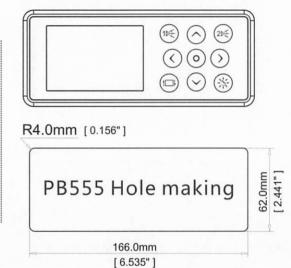
Make hole in the appropriate position on the tub. Keep the hole and its surrounding area clean. If there is burr around the hole, it has to be removed to avoid infirm sticking of the panel.
