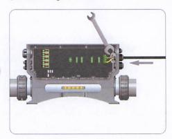
Plug the load power cable connector into the correspondent socket. Then reserve proper length for load power cable and tighten the glen head.
