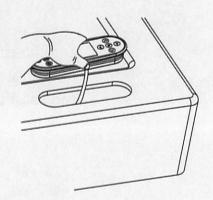
Press the panel for 30-60 seconds for firm sticking after placing it to the hole.
