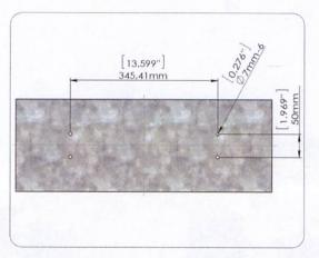
Make hole on the retaining plate as to the size and location descried in the graphic.
