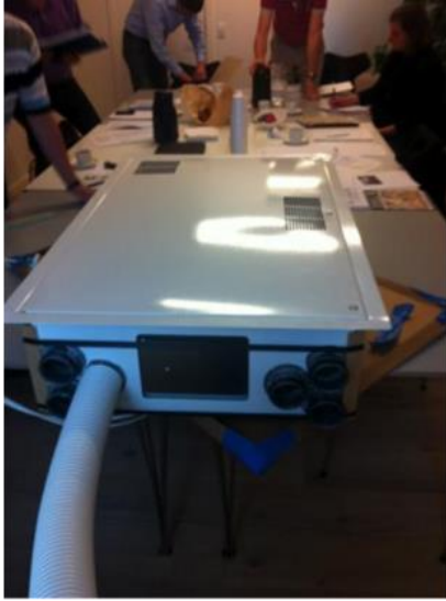
Compact HRV unit which can be roof or wall integrated
