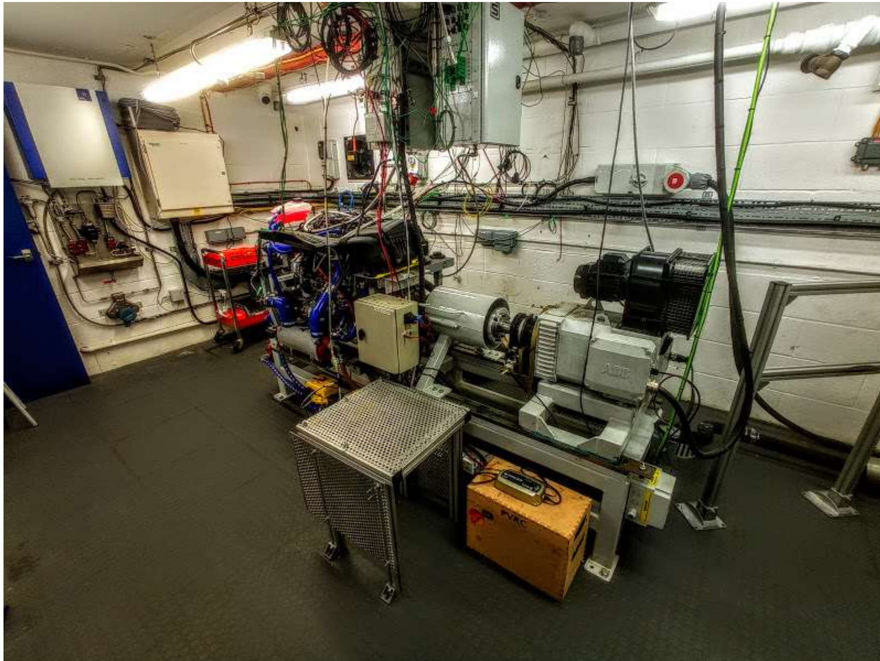
Photo 3 Ford Duratorq 2.0l Engine on ABB Engine Dynamometer
