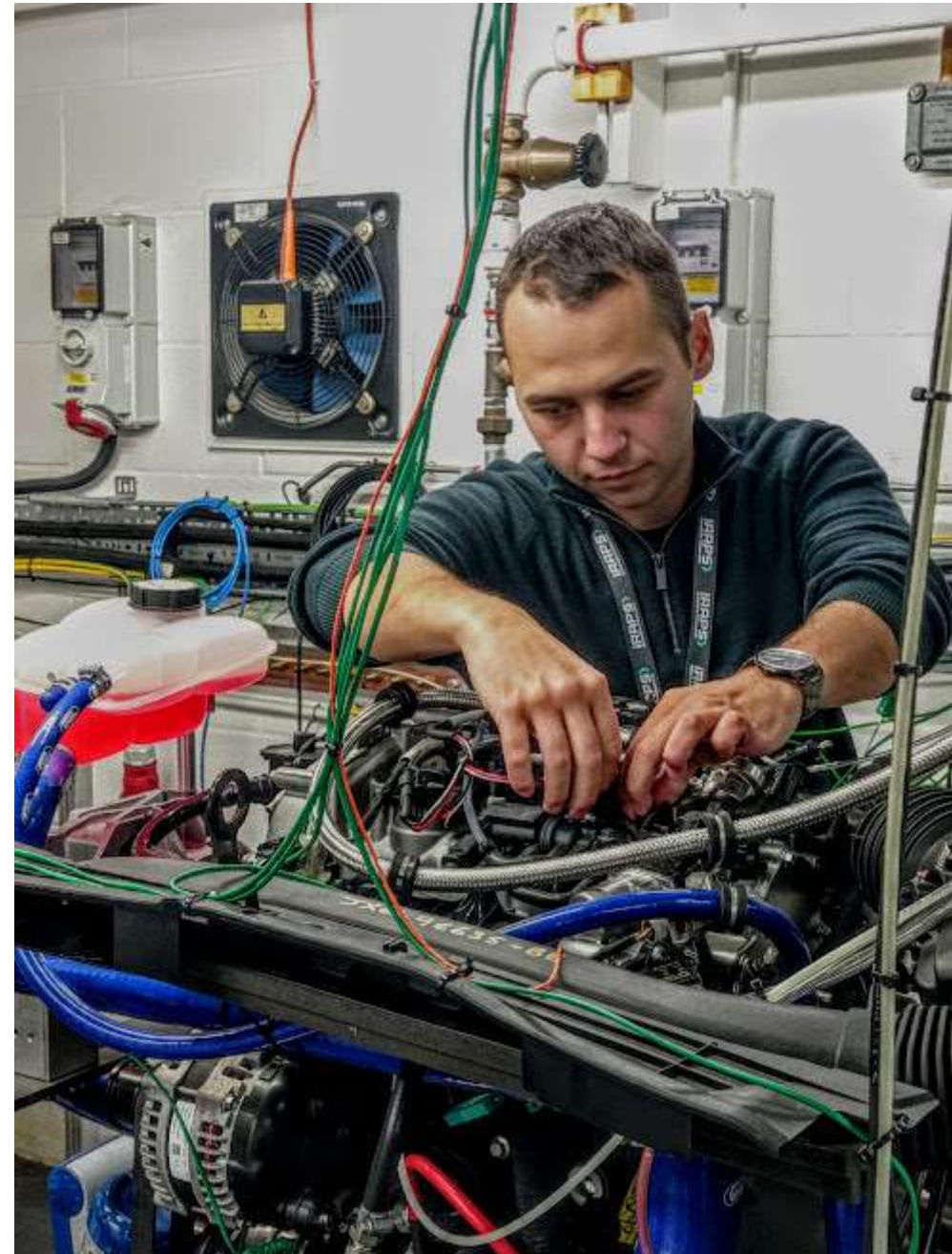
Photo 2 Connecting sensors to the engine
