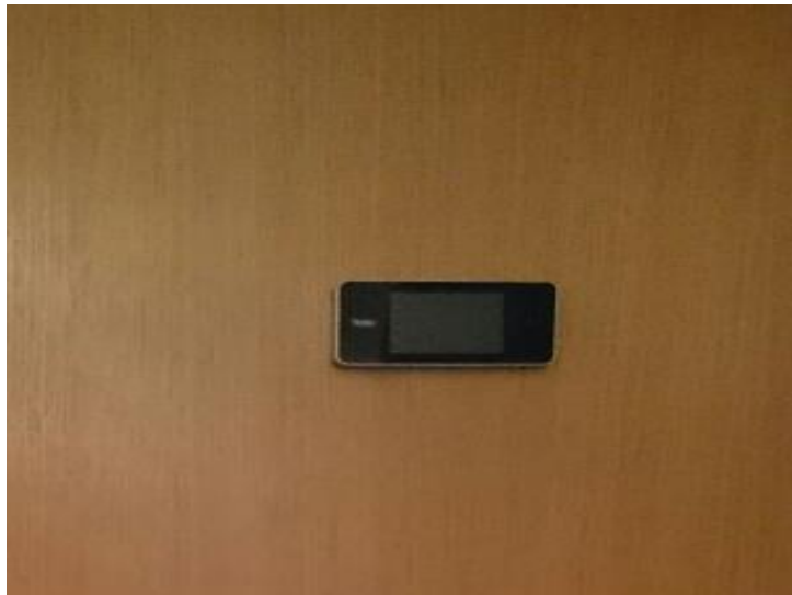
"Insidan" 1 tryckknapp AA-batterier
