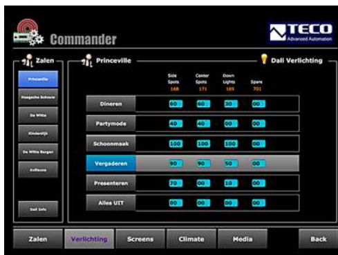
Lighting scene user setting. The final requirement is sent as a command to the subsystem delivered by Helvar.
