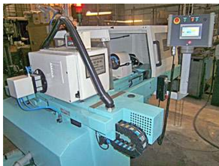
One of the first deployments of the GT-1753 positioning module utilized by KASKO company in Prague on automatic grinder BD 80 NC, which is used to grind cylindrical and conical holes in large series production.
