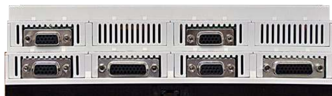
Four D-Sub15 connectors at the bottom are used to connect position sensors. Two D-SUB25 connectors use outputs ± 10V DC to control the actuator.
