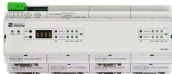
Module GT-1753 used to control 4 axes is designed in 12 modular box and attached to a DIN rail. The threaded green connector is used to connect the power supply and TCL2 system bus.
