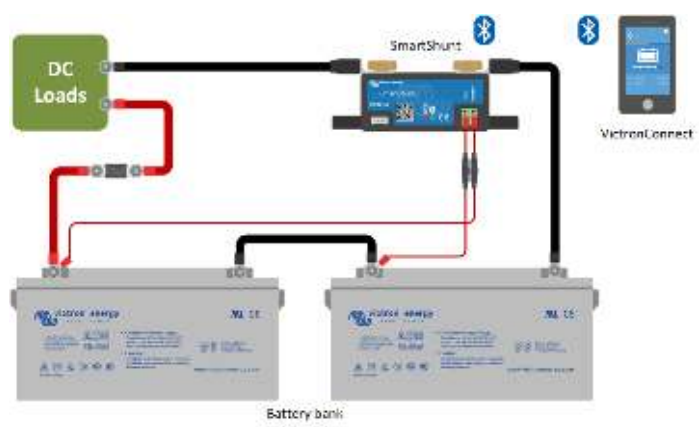
Measuring battery bank midpoint
