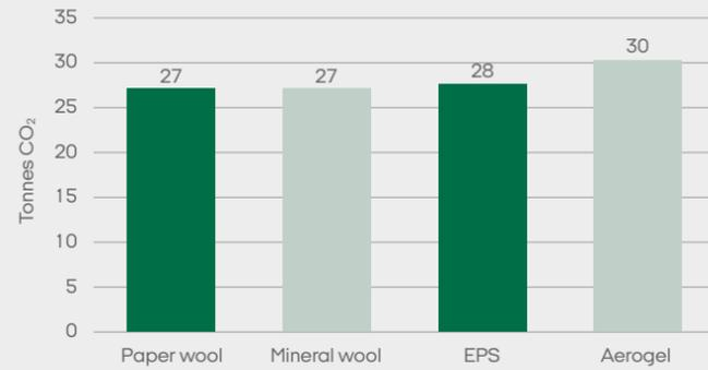
↑ CO<sub>2</sub> emissions from the restoration of Poul Henningsen's house based on a life cycle assessment. The "Aerogel" bar reflects the actual restoration, while the other bars show what the carbon footprint would have been if 2 cm of another insulation material had been fitted.
