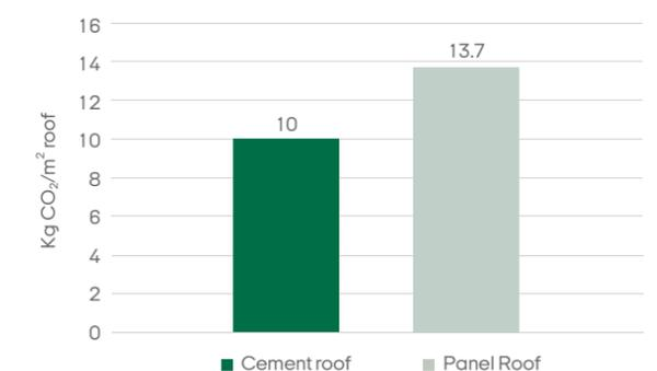
↑ The difference in CO<sub>2</sub> impact for the two types of roofing per square metre of roof.
