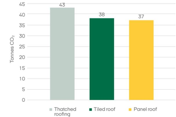
LCA for the whole restoration of Højgården on Sejerø with thatched roof compared with other types of roof. According to the LCA, five tonnes CO<sub>2</sub> more is emitted from a thatched roof than a tiled roof using the generic German EPD for tiled roofs. However, there can be great differences between the different types of roof, and using other, product-specific EPDs could turn things around completely.
