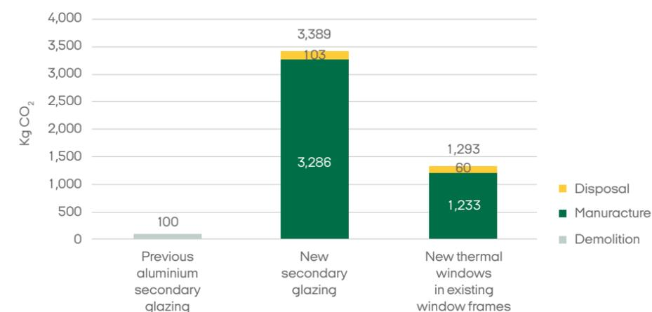
The carbon impact of restoring the windows in Edvard Heiberg's family house. The middle bar is the carbon cost of Realdania By & Byg's attempt to develop special secondary glazing for this and other functionalist buildings.
