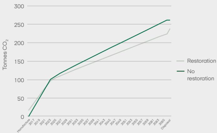
↑ CO<sub>2</sub>-emissions during and after the restoration vs. no restoration The graph shows how the overall restoration of Poul Henningsen's house generates long-term CO<sub>2</sub> benefits compared to no restoration [the break in the curves marks the transition from natural gas to direct heating in 2024].
