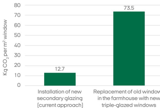
The graph shows the difference in CO<sub>2</sub> emissions from fitting new secondary glazing with wood frames in the farmhouse and the intended replacement of the old windows with new triple-glazed windows, including replacement of the wood frames. The figures shown are per m<sup>2</sup> window area.
