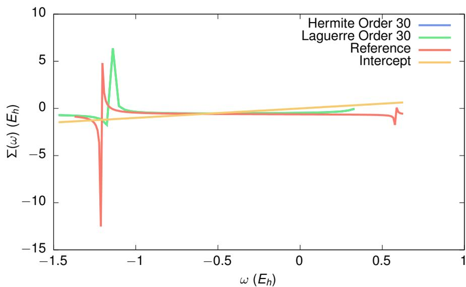
Figure 7.7: The plot shows the real part of the self-energy diagonal matrix element of the HOMO level of a hydrogen molecule. The results were computed by combining the COHSEX and the vertical integration approach. That way, the reference data can be reproduced very well. Especially the intercept is approximated very well as can also be seen from table 1.
