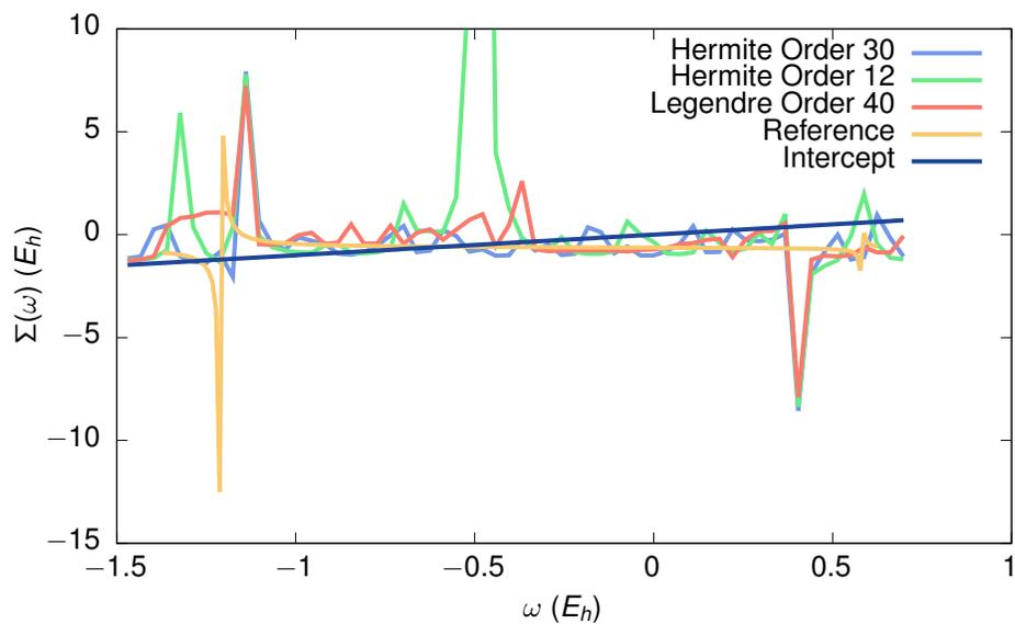
Figure 7.6: The plot shows the real part of the self-energy diagonal matrix element of the HOMO level of a hydrogen molecule. The results were computed using the COHSEX splitting approach and numerical integration along the real axis. It can be observed that compared to figure 7.2 the results are more stable when changing the quadrature. However, when the quadrature order is too small the accuracy of the results suffers as can be seen from the graph of the Hermite quadrature of order 12.
