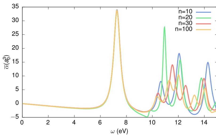
Figure 5.1: The graph shows the isotropic average of the polarizability tensor of benzene for different frequency grids. The first peak is reproduced for even small grids with only ten grid points. For frequencies larger than 10 a higher number of grid points is needed for better accuracy.
