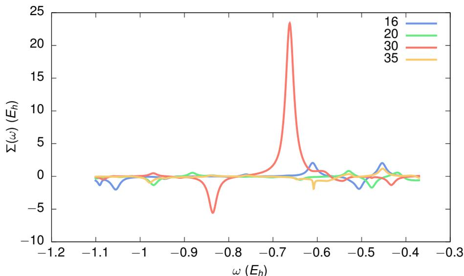
Figure 7.2: The plot shows the real part of the self-energy diagonal matrix element of the HOMO level of a water molecule. Different integration orders of the Gauss-Hermite quadrature were used to integrate along the real axis to produce these results. It can be observed that changing the quadrature order drastically changes the results. Consequently, integrating along the real axis is not a feasible option.
