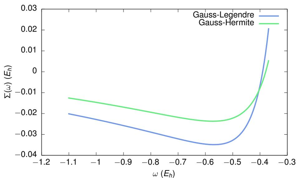
Figure 7.3: The plot shows the real part of the self-energy diagonal matrix element of the HOMO level of a water molecule. For this test, imaginary frequencies combined with the Padé-approximation were used to produce the results. The structure of the self-energy cannot be reproduced by this approach as the values are way too small and in comparison to results from the standard approach show, that this integration method is also not feasible.
