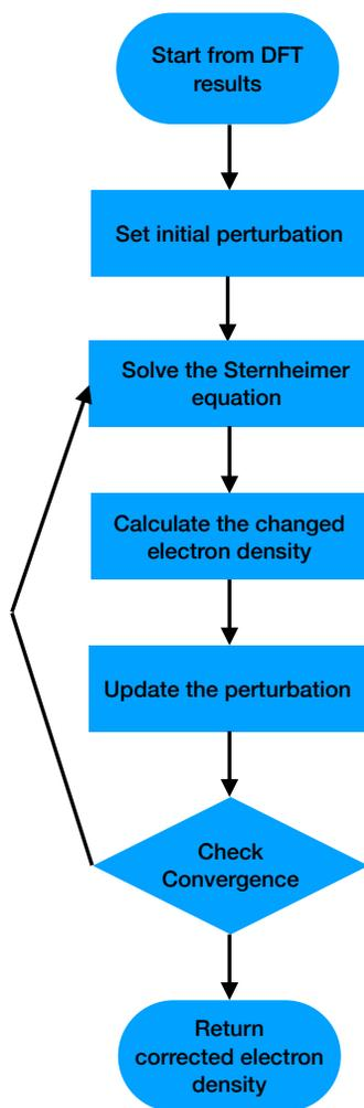
Figure 4.1: This flowchart describes the workflow of the self-consistent Sternheimer equation. In the following, each step is explained in detail.
