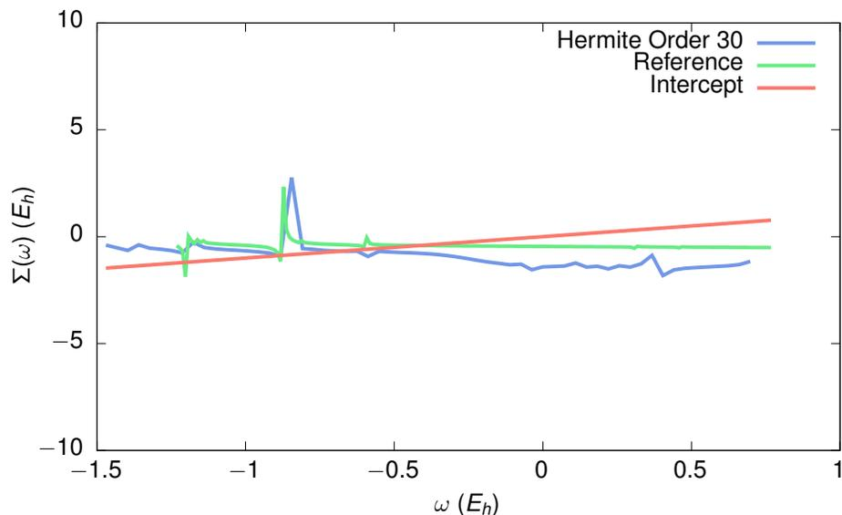
Figure 7.9: The plot shows the real part of the self-energy diagonal matrix element of the HOMO level of a water molecule. The result obtained with the *GW* Sternheimer is compared to the data produced using *votca xtp*. While the reference data could not be approximated as well as for Hydrogen, the structure of the plot is reproduced well. The intercept at  $-0.4142 E_h$  is only approximated as  $0.67 E_h$ .
