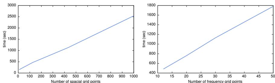
Figure 7.10: The plot shows the time needed to evaluate the *GW* Sternheimer method for Hydrogen for 10 frequencies, depending on the number of spatial grid points needed and the number of frequency grid points. The computation time depends linearly on the the number of grid points. A comparable computation using a standard *GW* approach used to obtain the reference results only took a few seconds.
