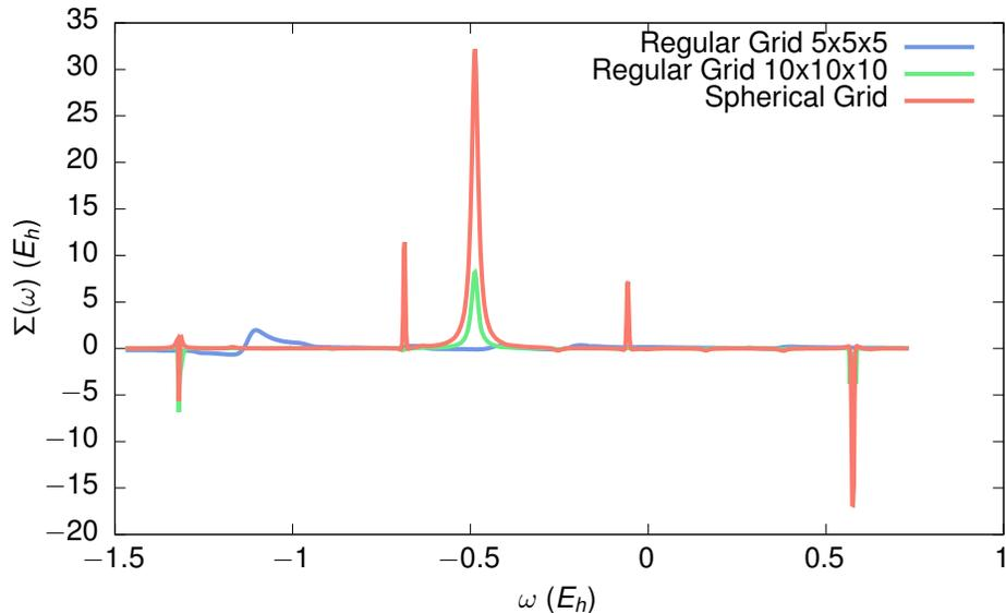
Figure 7.1: The plot shows the real part of the self-energy diagonal matrix element of the HOMO level of a hydrogen molecule. The grid with 5 points in each direction does not reproduce the results of the finer grids, whereas the spherical grid and the 10 step grid produce similar results. The peaks of the spherical grid graph are however much more pronounced although overall less grid points were used.
