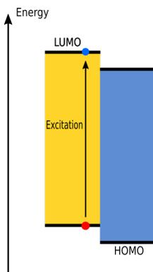
Figure 1.1: This figure shows the schematic structure of a two layer organic solar cell. In the left layer an electron is excited from the HOMO to the LUMO level, leaving behind a hole. The goal of this thesis is to implement an alternative way to obtain the excitation energy of an exciton like this. That in turn allows to find new materials that can be used in organic solar cells.
