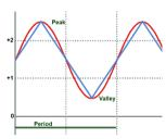
If input pulses derive from magnetic speed sensors the signal is generally sine with an equal positive and negative half (not offset as shown above). The BSL350 only measures and triggers on the positive part of an input signal these signals will have a valley equal to 0 and the peak equal to the highest  $VaPMek = \sqrt{12} \times V_{RMS}$  for a sine wave).
