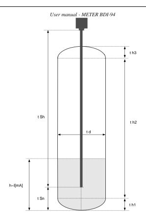
Figure 7.1 Parameters of cylindrical tank in vertical position.
