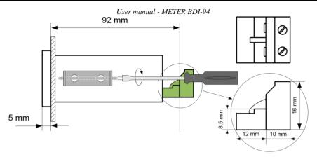
Figure 4.3. Installing of brackets, and dimensions of connectors.
