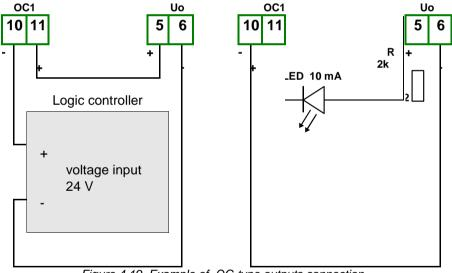
Figure 4.19. Example of OC-type outputs connection
