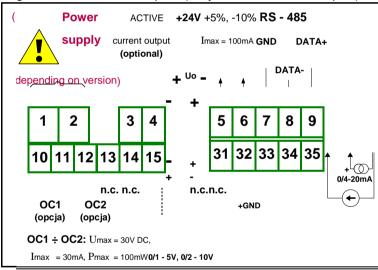
Figure 4.9. Terminals description (OC-type and active current outputs)
