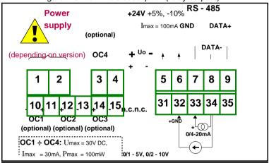
Figure 4.7. Terminals description (OC-type outputs)
