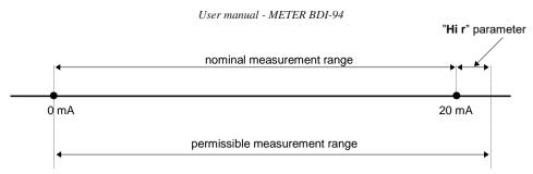
Figure 6.2. Definitions of measurement ranges in mode 0 ÷ 20mA
