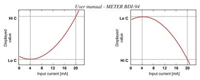
Figure. 10.2 Normal ("Lo C" < "Hi C) and inverted ("Lo C" > "Hi C) characteristic
