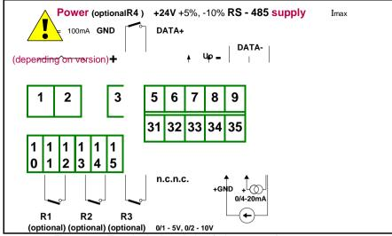
Figure 4.6. Terminals description (relay outputs)
