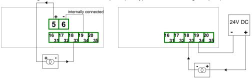
Figure 4.14. Connection of 2-wire current converters
