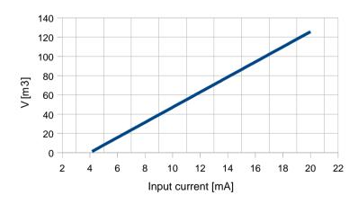
Figure 10.6 The volume characteristic of tank depending on input current in 4÷20mA range.
