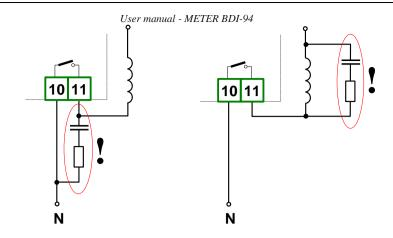
Figure 4.18. Examples of suppression circuit connection: a) to relay terminals; b) to the inductive load
