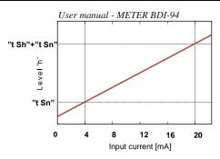
Figure 10.5 The characteristic of level of liquids, gases or solids in tank depending on input current in 4÷20mA range.
