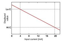
Figure. 10.1 Normal ("Lo C" < "Hi C) and inverted ("Lo C" > "Hi C) characteristic
