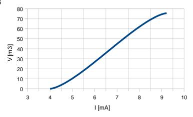
Figure 10.7 The volume characteristic of tank depending on input current in 4÷20mA range.
