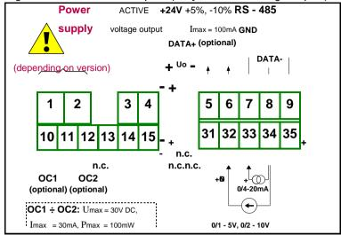
Figure 4.13. Terminals description (OC-type and active voltage outputs)
