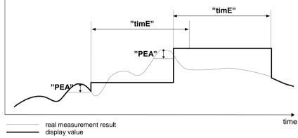
Figure 6.3. Process of peaks detection
