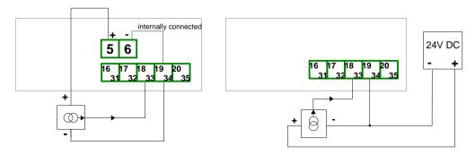
Figure 4.15. Connection of 3-wire current converters
