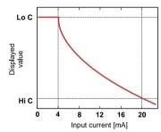
Figure. 10.3 Normal ("Lo C" < "Hi C) and inverted ("Lo C" > "Hi C) characteristic
