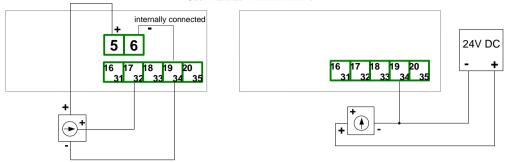
Figure 4.16. Connection of voltage converters
