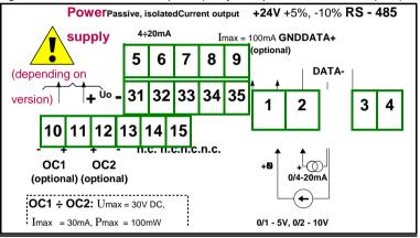
Figure 4.11. Terminals description (OC-type and passive current outputs)
