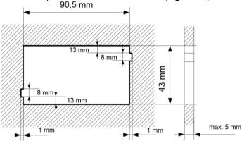
Figure 4.1. Recommended mounting hole dimensions 92
