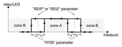
Figure 6.5. Two threshold control of the relay/LED outputs
