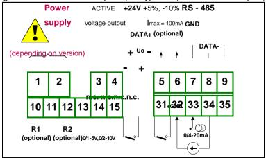
Figure 4.12. Terminals description (relay and active voltage outputs)
