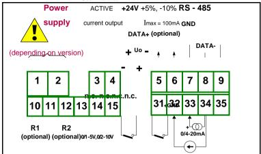
Figure 4.8. Terminals description (relay and active current outputs)
