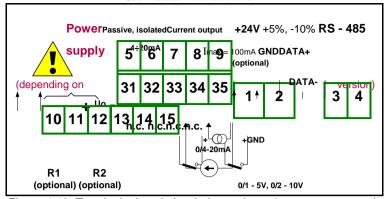
Figure 4.10. Terminals description (relay and passive current outputs)
