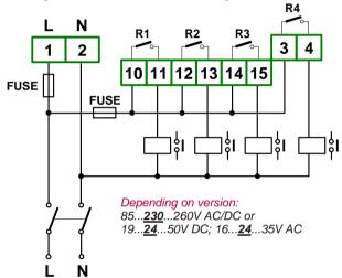
Figure 4.17. Connection of power supply and relays
