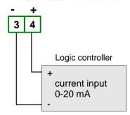
Figure 4.20. Example of active current outputs connection (for device with active current output only)
