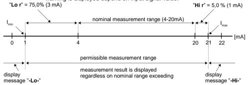
Figure 7.3 Example of definition of permissible range of input signal
