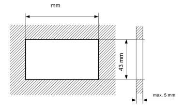
Figure 4.2. Allowable mounting hole dimensions
