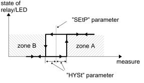
Figure 6.4. One threshold control of the relay/LED outputs
