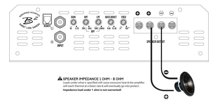
We recommend using minumum10 Ga speaker cables to acquire the intended performance & efficiency. Run the speaker cables from your speakers to the amplifier's mounting location.
