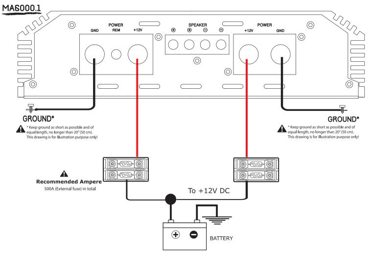
We recommend to use minumum10 Ga speaker cables to acquire the intended performance. Run the speaker cables from your speakers to the amplifier's mounting location.
