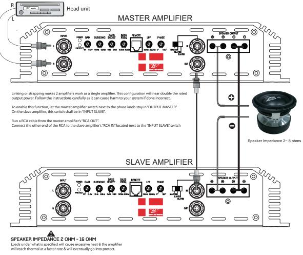
Strapped impedance load under 2 ohm is not warranted!
