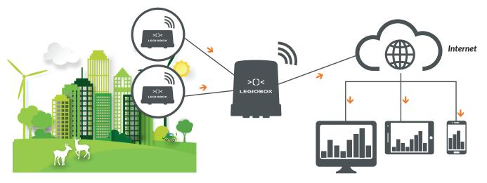
Energy, gas and water information is collected from the energy meters and sensors using the PicoWise and the NanoGate The NanoGate acts as GateWay and sends the data to the data center Internet NRGVision is the cloud-based platform that gives insight into your energy gas and water usage.
