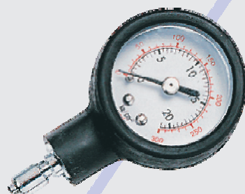
Line pressure, used to determine whether the free flow is a first or second stage problem
