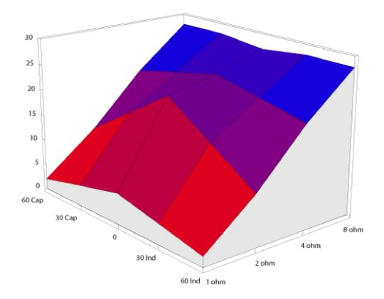
PowerCube graph of an amplifier with current limiting (image courtesy of AudioGraph AB).
