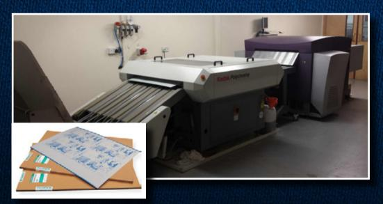
Computer To Plate (CTP) imaging technology is used in our modern printing processes. With this technology, we produce an image created in Desktop Publishing (DTP) application directly to a printing plate.
