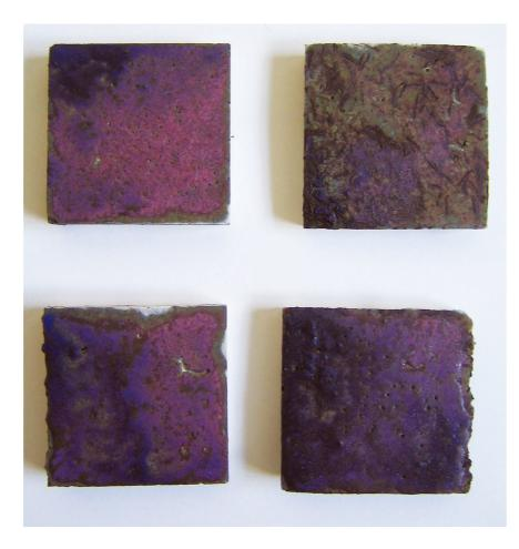
Glaze recipe 1 (light red-dark purple). Thin layer on the top left on Wearcast 2000 HT with no fibres and on the right with fibres. Bottom left, same glaze but with a thick layer, on the left no fibres and the right with fibres. Glaze fired 80 C°/H up to 1260 C° with a standing time of 30 minutes. Photo: Anja.
