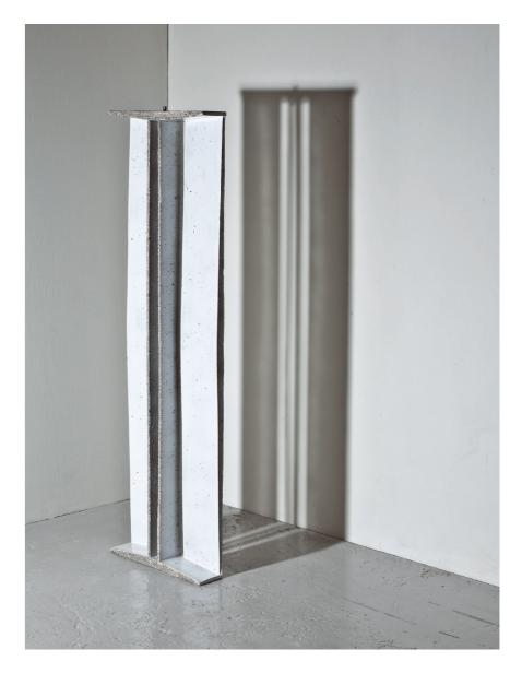
This and opposite page: self-supporting façade solutions made from specific ceramic glazed concrete with exposed and visible reinforcement barsand connector. 160 cm x 50 cm x 1-3 cm. Photo: Ole Akhøj.
