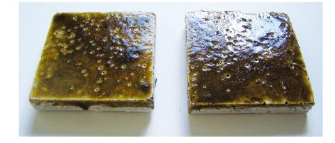
Top: Glaze recipe 2 (Turquoise-blue mat). Left on Wearcast 2000 HT with no fibres. On right with fibres. Glaze fired 80 C°/H up to 1260 C° with a standing time of 30 minutes. Bottom: Glaze recipe 3 (brown black). Left on Wearcast 2000 HT with no fibres, right with fibres. Glaze fired 80 C°/H up to 1260 C° with a standing time of 30 minutes. There are holes in the surface of the object that the glaze here does not offset. Photo: Anja.
