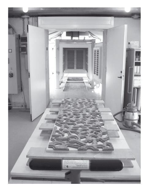
perature, which in my case is in the high range. This is necessary because the specific ceramic glazed concrete I use is densely packed. With a slow rise in temperature, 50 C°/H, I ensure that free water bound within the other ingredients can be released without the risk of explosion. In densely packed concrete, the water might have a difficult time being released from the concrete.
