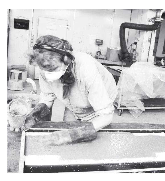
ntally and level when level plates are desired. These can then subsequently be assembled with jointing and thusly be transformed into spatial objects. It is, however, also possible to make a mould that when it is de-moulded produces the desired spatial object without utilizing jointing. There are advantages and disadvantages to both methods. Which method to use depends much on the form and expression the object is meant to have. In the following I go over both methods.
