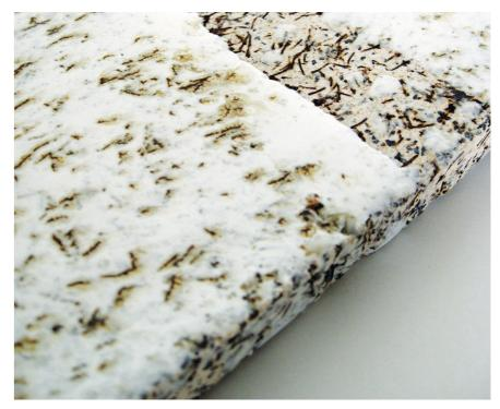
Top: mix 50% glaze recipe 1 mixed with 50% glaze recipe 2. Left on Wearcast 2000 HT with fibres and on the right no fibres. Glaze fired 80 C°/H up to 1260 C° with a standing time of 30 minutes. On the right Ceramas white, glossy stoneware glaze 1302 on Wearcast 2000 HT with fibres. Glaze fired 80 C°/H up to 1260 C° with a standing time of 10 minutes. Photos: Anja.
