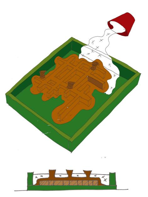
This lubricant is made from stirring and heating soap flakes in water, melting the soap flakes. The corn oil is mixed into this. The mixture is then set somewhere cool, and acquires a solid, yet greasable consistency, much like cool butter. In some cases, it might be a good idea to grease both the positive mould and the surrounding wooden mould with W40, either to replace or supplement the soap-oil mixture. This should be a thin layer with no pools.
