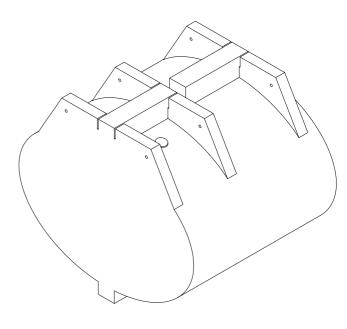
In case of foamed pontoons, 2 additional plugs are present on the float
