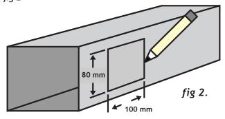
5. Cut out the traced portion of the duct using snips or sheet metal cutters. fig 3
