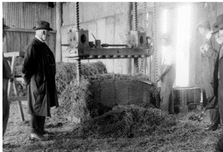
Hay Baler inspected by 1910 Scottish Agricultural Commission visit to Tocal, Paterson. (Tocal archives). Note the gear box to allow operation by horse works.
