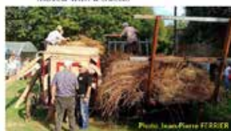
Threshing with a threshing machine moved with a tractor
