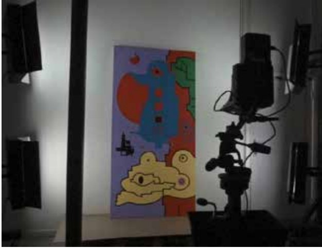
Fig 2 Linhof Master Technik classic Camera 4x5 / Anagram production2 312Mp / 4x Fluorescent light Type 6 6 x 55 Watt
