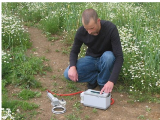
Measuring soil respiration in the field, February 2014 by Steveaduck, Creative Commons
