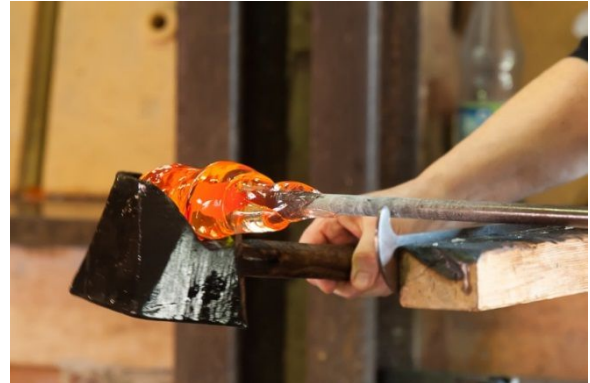
Hand-shaping glass with the aid of the wooden instrument called a Wulgerholz in German, Photo LWL/Tegeler
