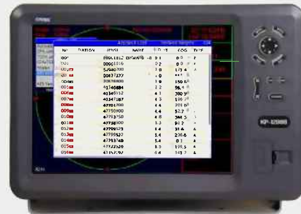
Built-in Class B AIS Receiver
