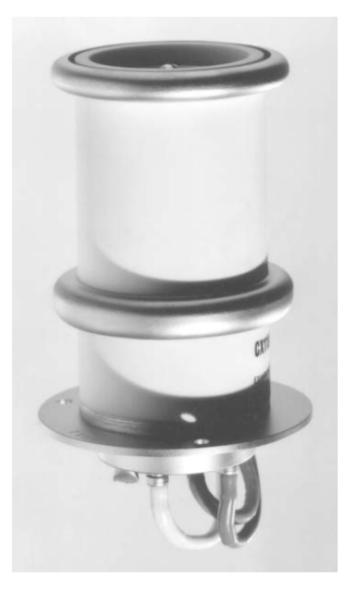
The cathode end of the tube must be cooled whenever heater voltages are applied, since the cathode flange will reach a temperature of 120 °C above ambient in the absence of cooling. Envelope temperature:
