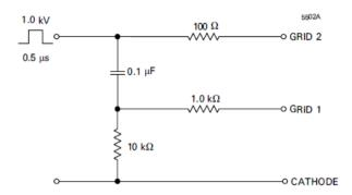
Fig. 1 Circuit for single pulse drive
