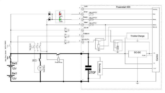
This block diagram is showing a typical (parallel) configuration. Configuration may vary per application. A dedicated start configuration is also possible.
