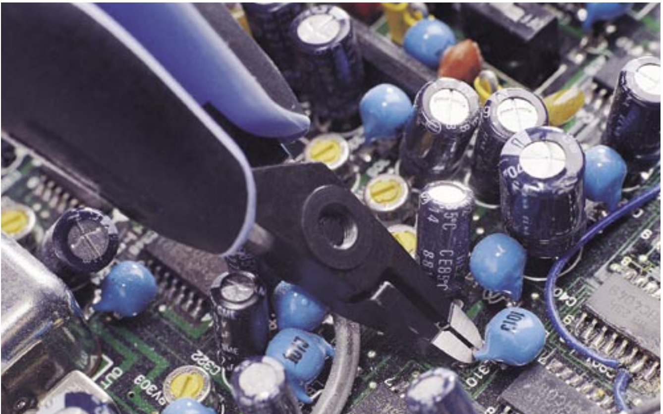
Tip cutter Rx8149 is an even more specialized adaptation of the tapered and relieved style. Its extreme tapering on all sides allows access and reach. See page 42 for more on Rx8149.
