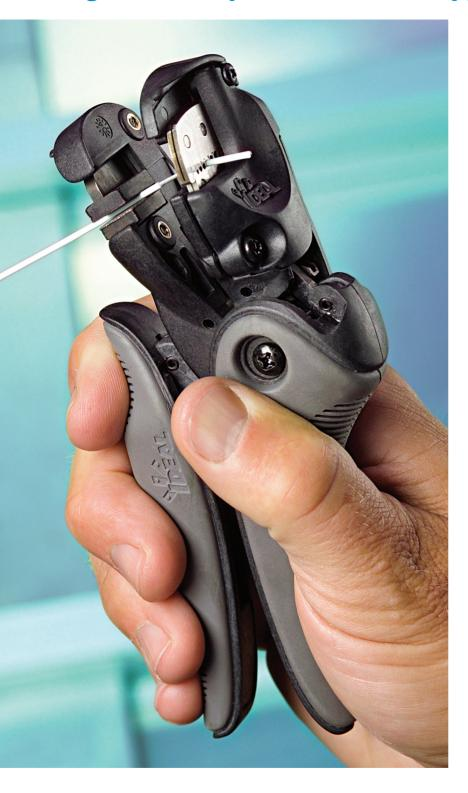
IDEAL has set the aviation industry's standard in handheld, precision wire stripping for over 60 years. IDEAL is known for it's innovative one-step squeeze-action stripper and patented blade design.
