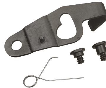
Short-stop Latch protects wire strands by limiting the stripping stroke to \frac{5}{32} in. and retains the slug until the wire is ready for terminating.
