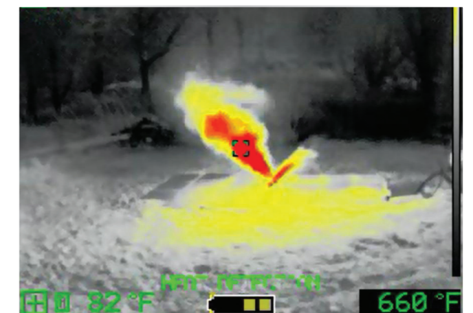
Invisible gas detected by the Mi-TIC
