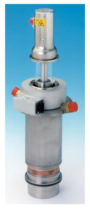
The magnetron output window may be cooled by either high pressure air or an arc suppressant gas such as  $SF_6$ . When the output window is cooled by high pressure air, a flow of not less than 0.085 m³/minute (NTP) into the air inlet at the base of the launching section is required. If  $SF_6$  is used, then no gas flow is required to cool the window. See note 7.
