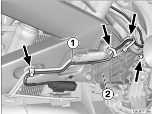
Remove the original cable ties (arrows) and re-secure connecting line
