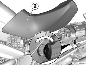
• Turn the key counter-clockwise (detail) and remove front seat (2).
