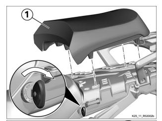
• Turn the key clockwise (detail) and remove rear seat (1).
