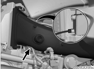
Check that the throttle-valve cable is seated in the guide of the air intake pipe (arrow) and that it is has not been pulled out of the divider (detail).
