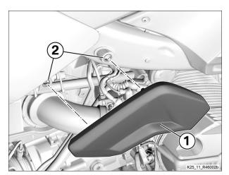
• Unclip side cover (1) from holders (2) and remove.
