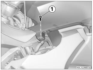
• Remove screws (1) on left and right.
