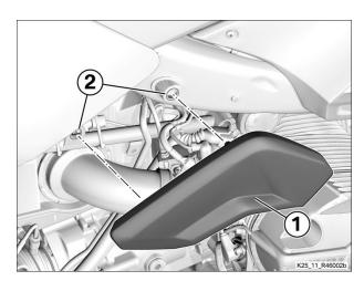
Hold side cover (1) in position and push the snap-fit studs into holders (2).
