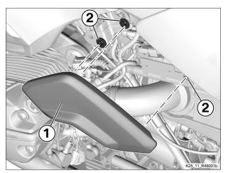
• Unclip side cover (1) from holders (2) and remove.
