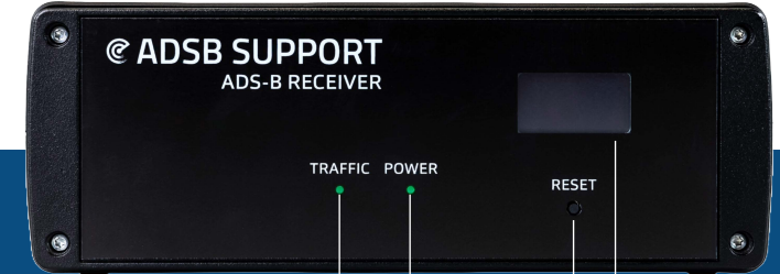
Traffic LED Power LED Reset button OLED screen
