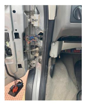
STEVE H SENT THE PHOTOGRAPH ABOVE OF THE WIRING REPAIR HE WAS FORCED TO UNDERTAKE AFTER HIS CENTRAL LOCKING AND WINDOWS STOPPED OPERATING. THE WIRES IN THE DOOR HINGE AREA HAD BECOME SEVERED AFTER YEARS OF CONSTANT USE.
