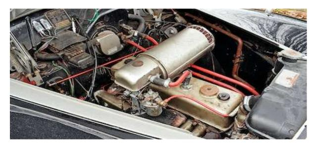
THE ENGINE BAY IS PRESENTABLE WITH NO LEAKS, THOUGH THE BRIGHT RED METAL PIPEWORK WON'T PLEASE PURISTS. BOTH THE BULKHEAD AND INNER WINGS APPEAR TO BE FREE FROM CORROSION. IGNITION COIL AND HT LEADS APPEAR TO BE RECENT ADDITIONS AND THE ELECTRICS HAVE BEEN CONVERTED TO NEGATIVE EARTH.
