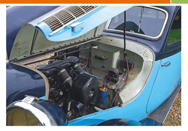
THIS 326'S 1971CC BRISTOL 85A ENGINE WAS FITTED IN SEPTEMBER 1948
