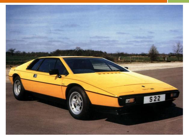
THE FIRST SERIES OF ESPRIT HAD BEEN FITTED WITH STANDARD WHEELS BY WOLFRACE WHICH TENDED TO MAKE THE CAR LOOK A BIT TOO REMINISCENT OF LOTUS "KIT CAR" ORIGINS. TO BE IN THE PORSCHE CLASS THE ESPRIT NEEDED CUSTOM WHEELS AND FOR THE SERIES 2 IT WAS GIVEN THEM. THE NEW CUSTOM WHEELS WERE MADE FOR LOTUS BY ITALIAN COMPANY SPEEDLINE AND THEY HELPED TRANSFORM THE LOOK OF CAR UP INTO THE CLASS THAT IT WAS INTENDED FOR.
