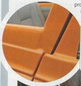
Strengthen The cavity along the side windows is filled with a 2mm folded plate and welded, giving extra strength.
