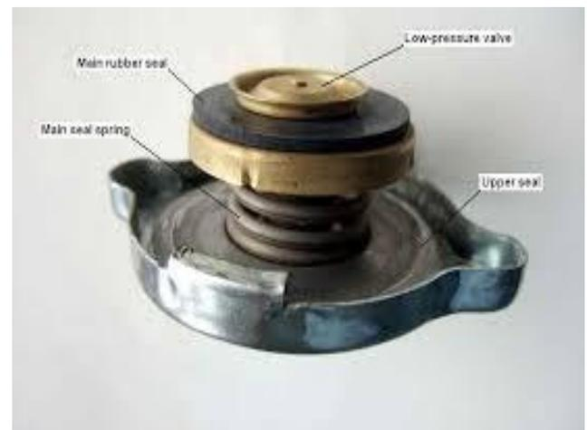
Check the main rubber seal. It should be free from cracks and be flexible. The seal together with the main spring keeps the system pressurised. Any faults here and you will lose water and overheat.
