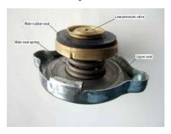
Check the main rubber seal. It should be free from cracks and be flexible. The seal together with the main spring keeps the system pressurised. Any faults here and you will loose water and overheat.
