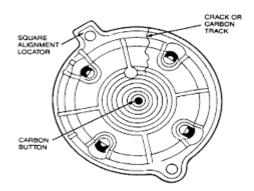
Check the terminals for erosion and 'gauging' also carbon build up. Excessive gap / resistance between rotor arm and terminal will reduce the power of the spark when it arrives at the plug gap. The golden rule is 'if in doubt, renew the cap'.
