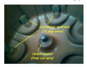
The carbon bush, or button, inside contacts the rotor arm. Many are spring loaded; check that the bush doesn't 'wobble' in the cap and it is free to move on its spring. Some bushes are of a fixed type in the cap (the rotor arm will have a spring loaded blade to make the contact). Check the bush is secure and not loose. They have been known to fall out when the cap is removed.
