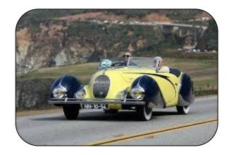
The 1938 Talbot Lago T150SS must be one of the most graceful Art Deco inspired cars, with coachwork design by the French firm Figoni and Falschi. Only a handful were made and prices are eyewatering. The engine was a 140 bhp, 3,996 cc inline six-cylinder engine with triple Stromberg carburettors.
