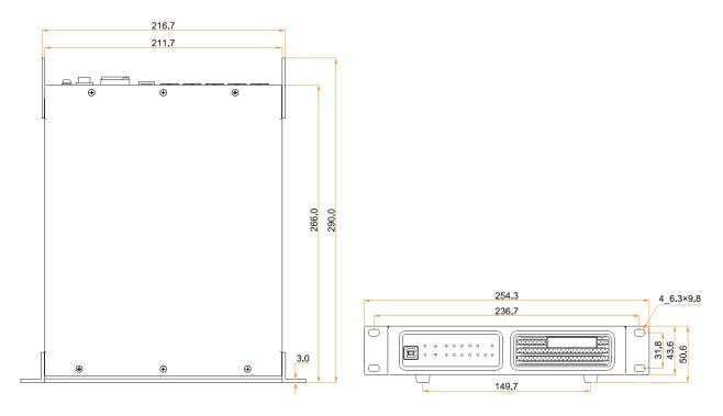
Tolerance: ±0.3 Unit: mm
