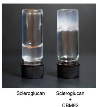
Figure 1. A hydrogel forms spontaneously when a CBM protein is mixed with scleroglucan in water at room temperature. No chemical modification of the polysaccharide is required to initiate this interaction.
