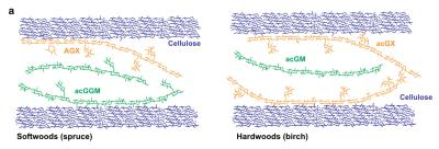
Schematic illustration of the polymeric network in a model BC-H system mimicking the secondary cell walls of softwoods and hardwoods prior to lignification. Ref: Vilaplana et al. Nature Communications 2020, 11, 4692
