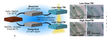
Transparent wood biocomposites by fast UV-Curing for reduced light-scattering through wood/thiol-ene interface design. Ref: Berglund, Johansson et al. ACS Appl. Mater. Interfaces 2020, 12, 41, 46914-46922.
