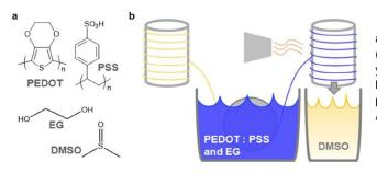
a) Chemical structures of PEDOT:PSS, EG, and DMSO. (b) Schematic of the yarn-dyeing process: the pristine yarn travels through the dye bath and is then dried by a heating gun and collected. Afterward, the coated yarn is post-treated with DMSO. (Ref: Müller, Hamedi et al. ACS Appl. Mater. Interfaces 2020,12, 56403-56412.
