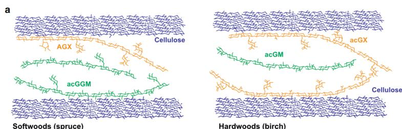
Schematic illustration of the polymeric network in a model BC-H system mimicking the secondary cell walls of softwoods and hardwoods prior to lignification. Ref: Vilaplana et al. Nature Communications 2020, 11, 4692
